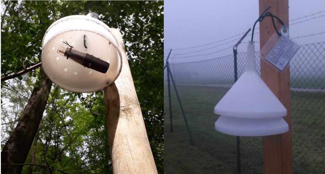
Figure 4: Lascar logger with a self-made double radiation shield, made from two white funnels. The inner funnel has holes to stimulate air flow. Pictures from Pieter De Frenne
