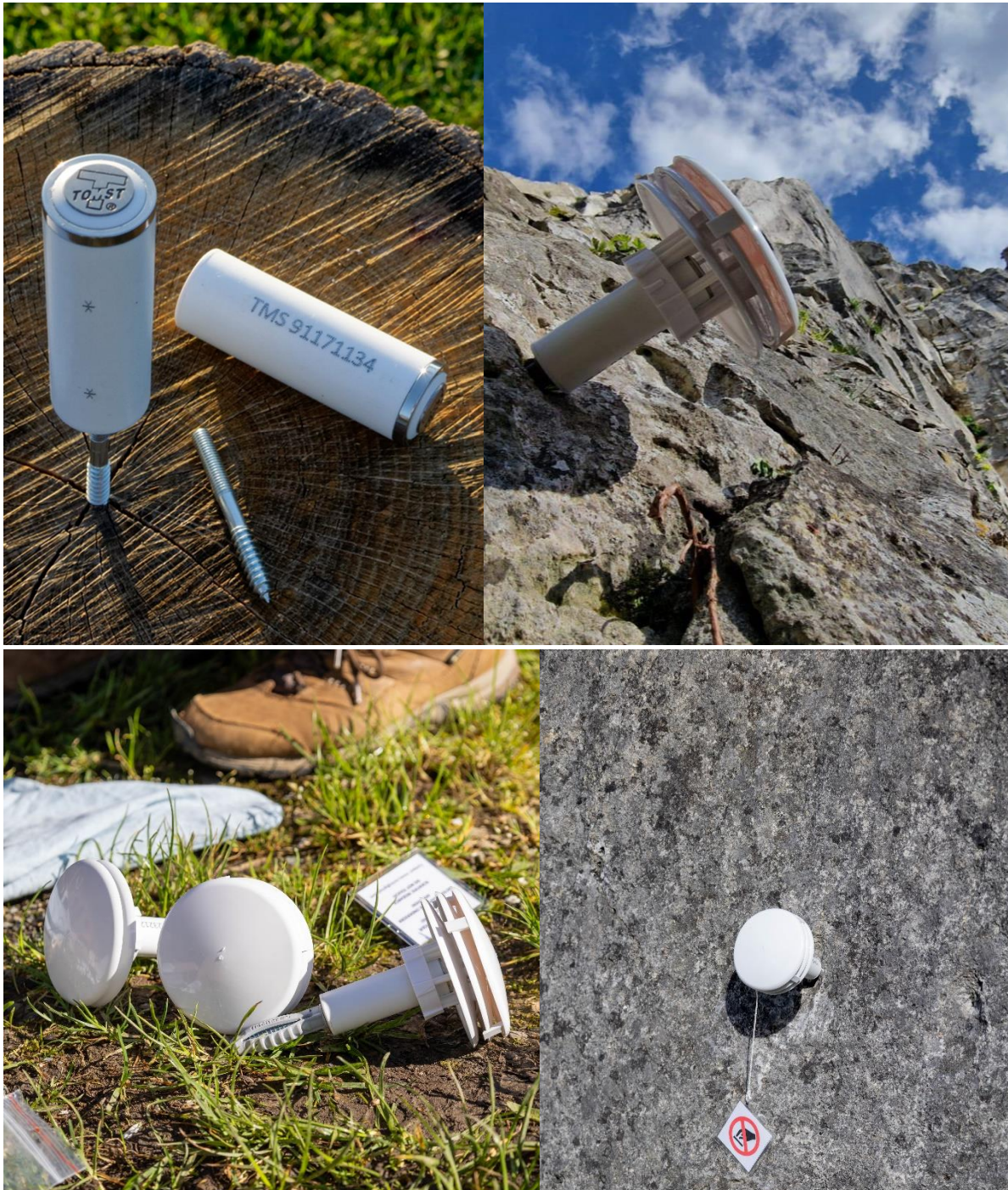
Figure 3: TOMST Thermologger can be used to measure the temperature at the rockface, as it comes with a handy screw and triple radiation shield. Pictures from https://tomst.com/ , Jonas Lembrechts and Kobe Burdack
